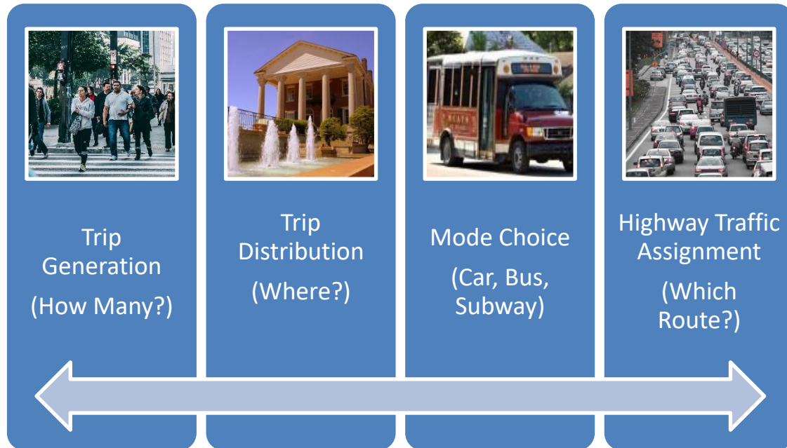
Figure 7 Four Step Travel Demand Modeling Process
